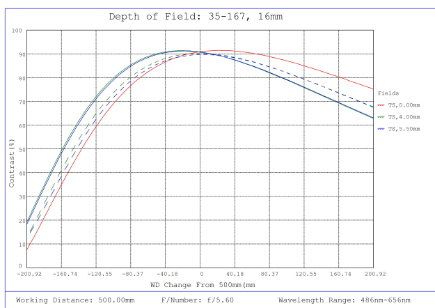
#35-167, 16mm, f/5.6 Cr Series Fixed Focal Length Lens, Depth of Field Plot, 500mm Working Distance, f5.6
