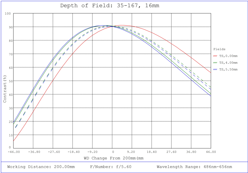
#35-167, 16mm, f/5.6 Cr Series Fixed Focal Length Lens, Depth of Field Plot, 200mm Working Distance, f5.6
