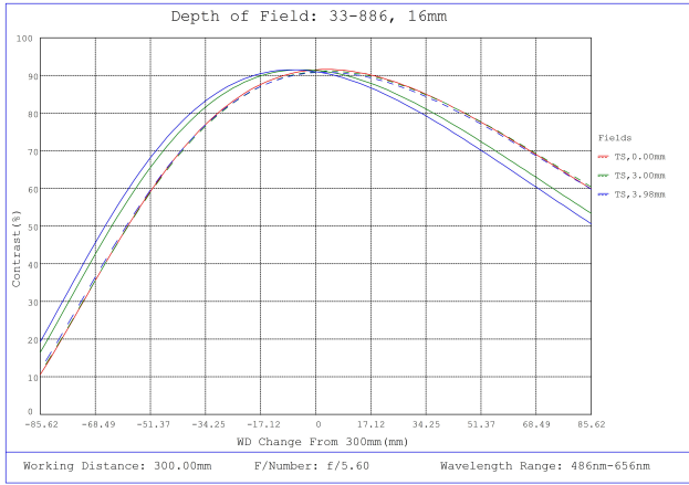
#33-886, 16mm, f/5.6 UCI Series Fixed Focal Length Lens, Depth of Field Plot, 300mm Working Distance, f5.6
