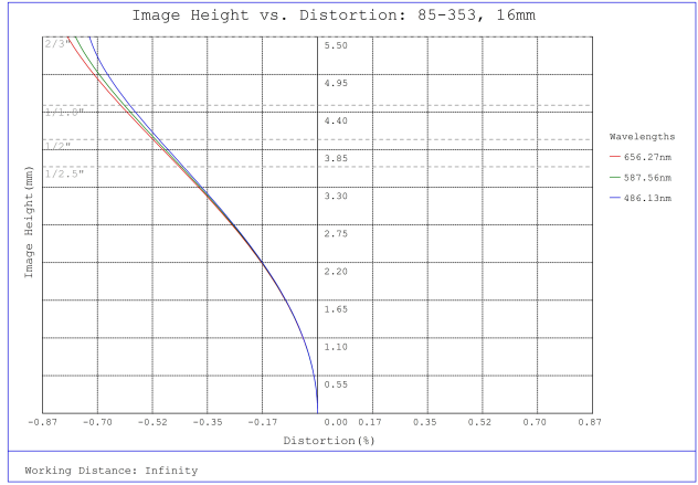
#85-353, 16mm, f/8 Ci Series Fixed Focal Length Lens, Distortion Plot
