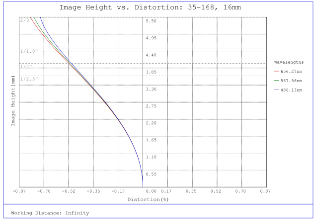
#35-168, 16mm, f/8 Cr Series Fixed Focal Length Lens, Distortion Plot
