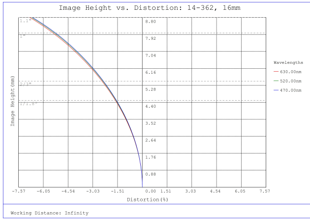
#14-362, 16mm LT Series Fixed Focal Length Lens, Distortion Plot
