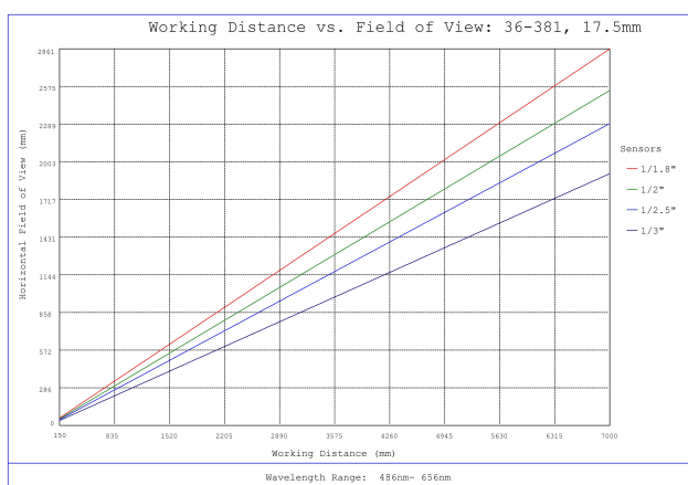
#36-381, 17.5mm FL f/4 , Rugged Blue Series M12 Lens, Working Distance versus Field of View Plot
