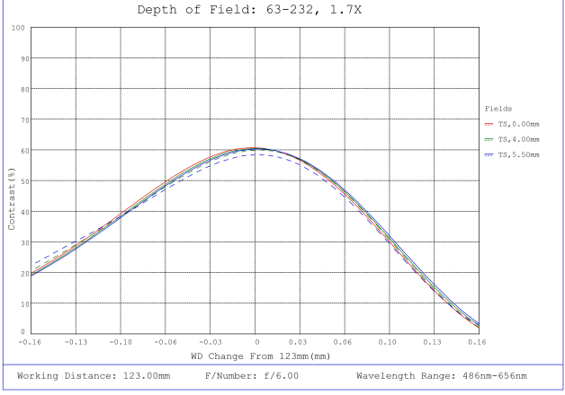
#63-232, 1.7X, 2/3" C-Mount PlatinumTL™ Telecentric Lens, Depth of Field Plot, 123mm Working Distance, f6
