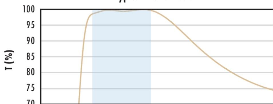
Typical transmission of a 3mm thick N-BK7 window with VIS 0° (425-675nm) coating at 0° AOI.
