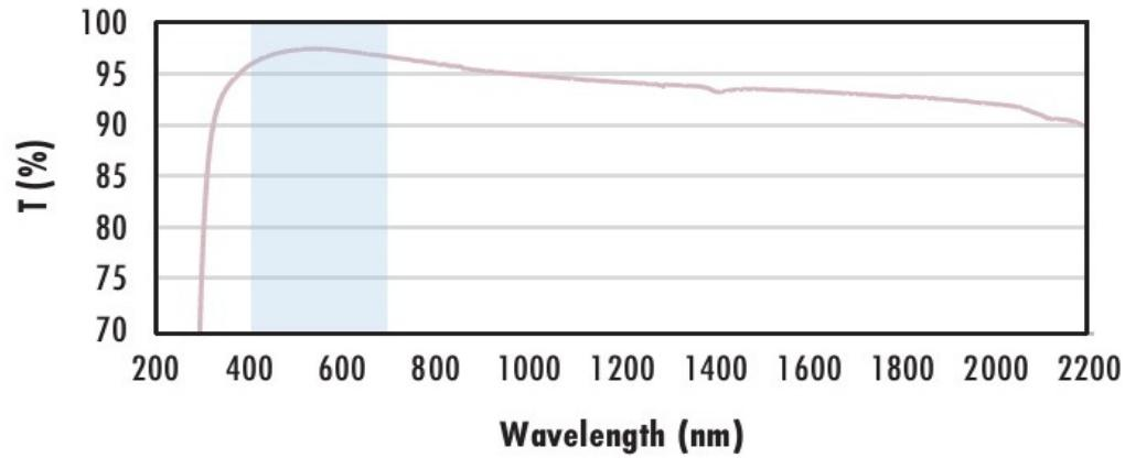
Typical transmission of a 3mm thick N-BK7 window with  $\text{MgF}_2$  (400-700nm) coating at 0° AOI.
