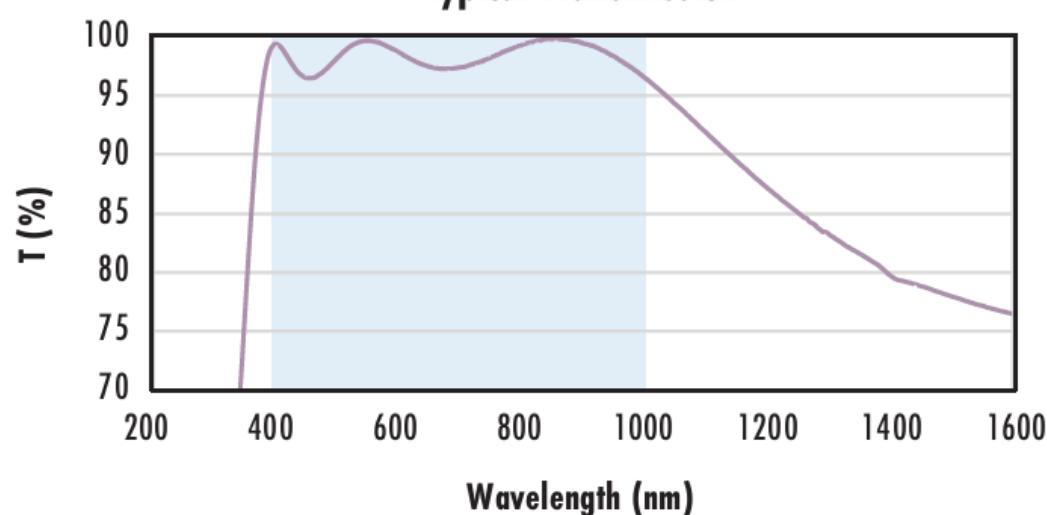
Typical transmission of a 3mm thick N-BK7 window with VIS-NIR (400-1000nm) coating at 0° AOI.
