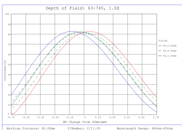
#63-745, 1X, 40mm WD CompactTL™ Telecentric Lens, Modulated Transfer Function (MTF) Plot, 40mm Working Distance, f11
