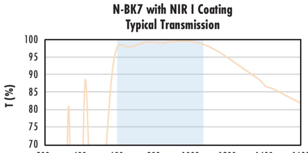
Typical transmission of a 3mm thick N-BK7 window with NIR I (600 - 1050nm) coating at 0° AOI.
