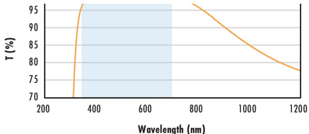
Typical transmission of a 3mm thick N-BK7 window with VIS-EXT (350-700nm) coating at 0° AOI.
