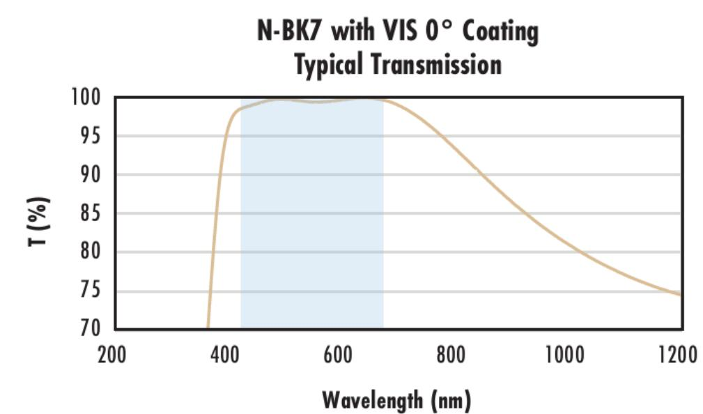
Typical transmission of a 3mm thick N-BK7 window with VIS 0° (425-675nm) coating at 0° AOI.
