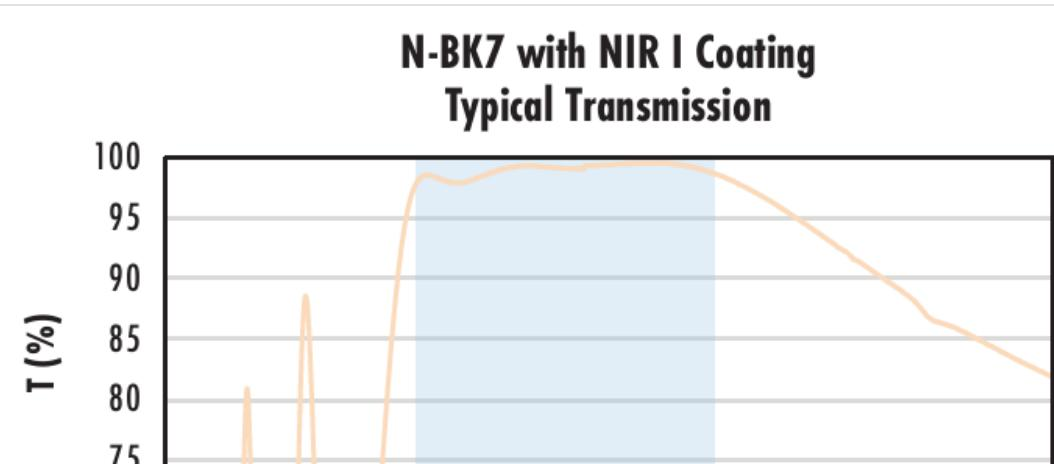
Typical transmission of a 3mm thick N-BK7 window with NIR I (600 - 1050nm) coating at 0° AOI.
