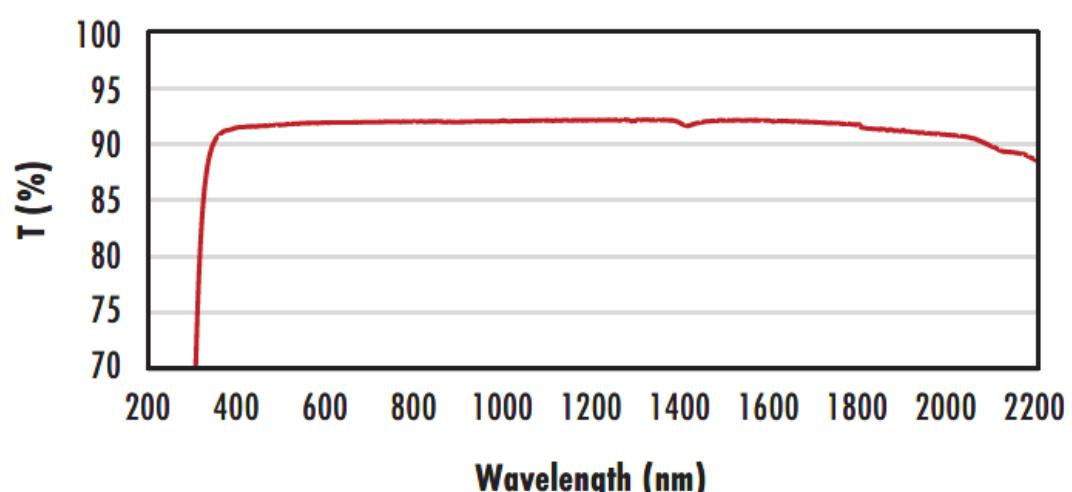
Typical transmission of a 3mm thick, uncoated N-BK7 window across the UV - NIR spectra.
