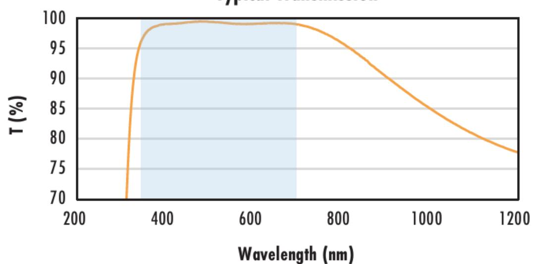
Typical transmission of a 3mm thick N-BK7 window with VS-EXT (350-700nm) coating at 0° AOI.
