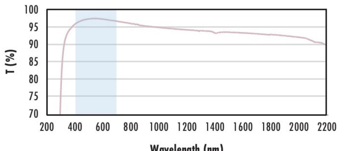
Typical transmission of a 3mm thick N-BK7 window with MgF<sub>2</sub> (400-700nm) coating at 0° AOL.
