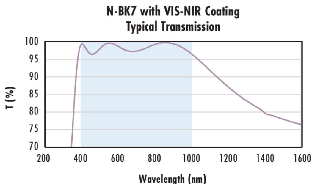
Typical transmission of a 3mm thick N-BK7 window with VIS-NIR (400-1000nm) coating at 0° AOI.
