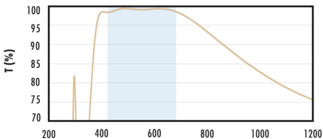
Typical transmission of a 3mm thick fused silica window with VIS 0° (425-675nm) coating at 0° AOI.
