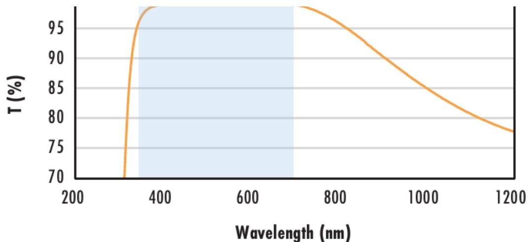
Typical transmission of a 3mm thick N-BK7 window with MS-EXT (350-700nm) coating at 0° AOI.
