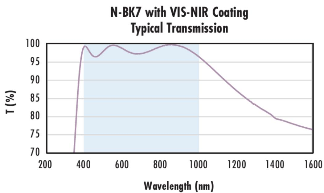
Typical transmission of a 3mm thick N-BK7 window with MS-NIR (400-1000nm) coating at 0° AOI.
