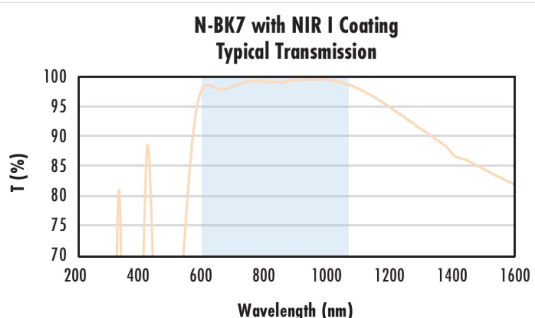
Typical transmission of a 3mm thick N-BK7 window with NIR I (600 - 1050nm) coating at 0° AOI.
