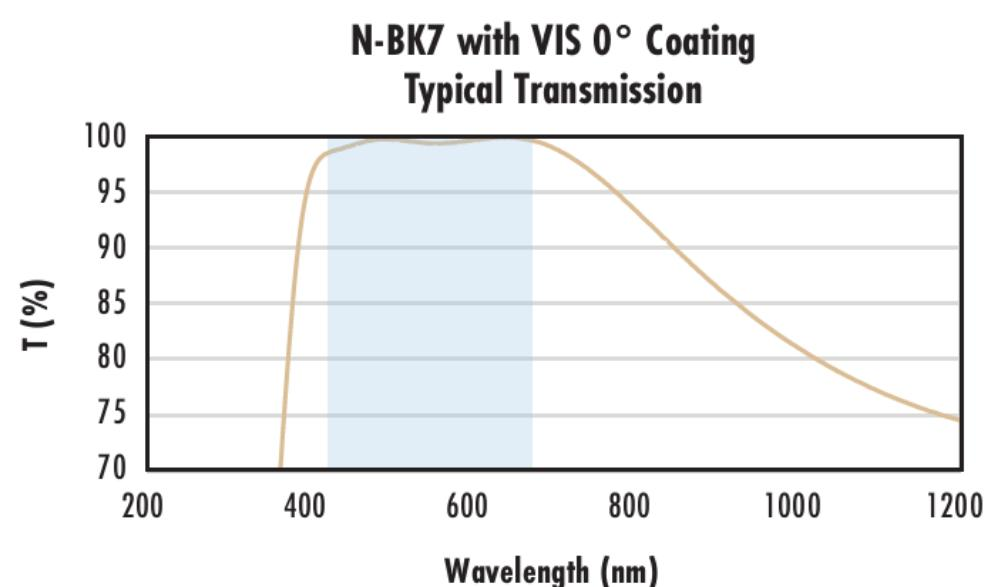
Typical transmission of a 3mm thick N-BK7 window with VIS 0° (425-675nm) coating at 0° AOI.
