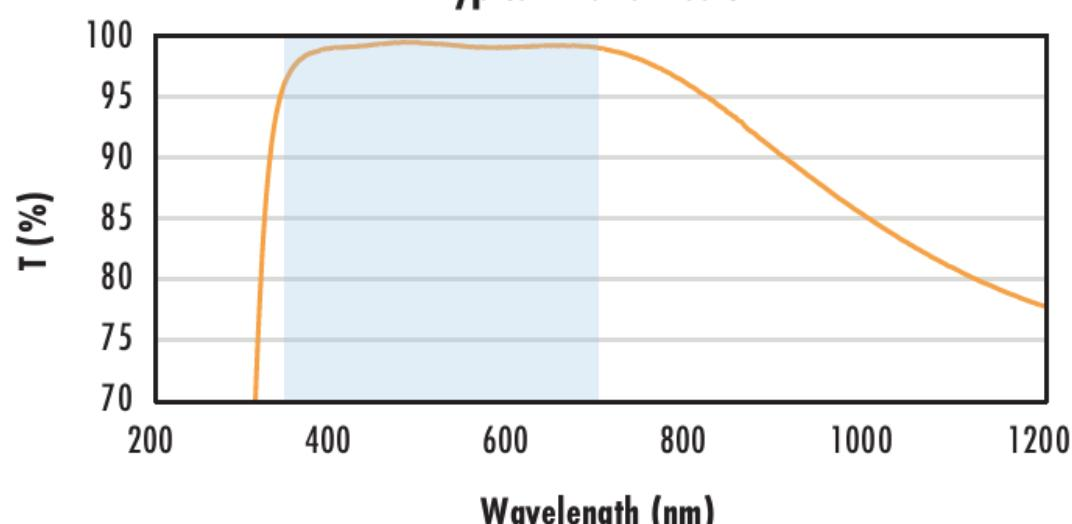
Typical transmission of a 3mm thick N-BK7 window with VIS-EXT (350-700nm) coating at  $0^\circ$  AOI.
