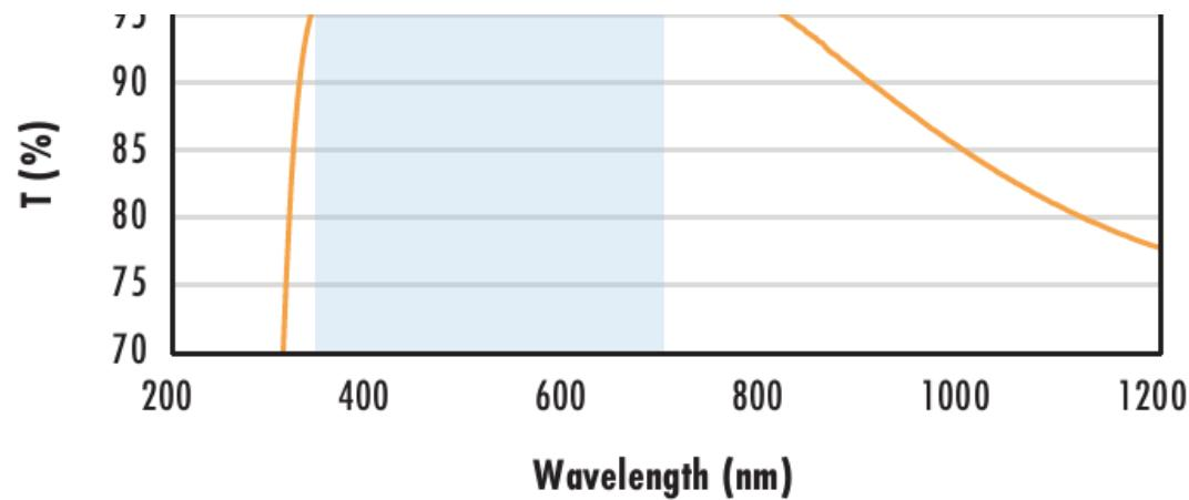
Typical transmission of a 3mm thick N-BK7 window with VIS-EXI (350-700nm) coating at 0° AOI.
