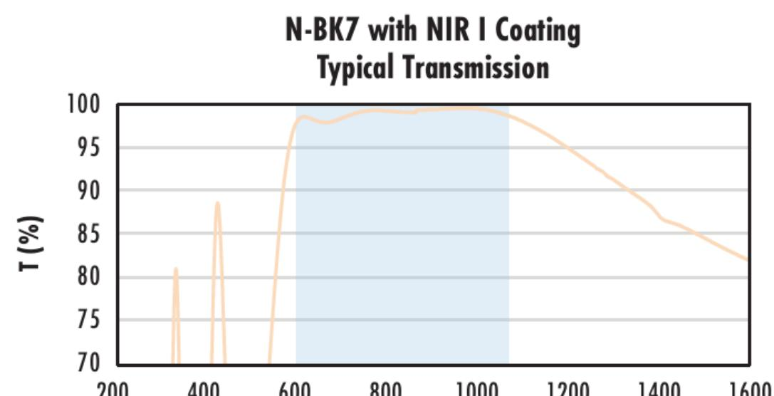
Typical transmission of a 3mm thick N-BK7 window with NIR I (600 - 1050nm) coating at 0° AOI.
