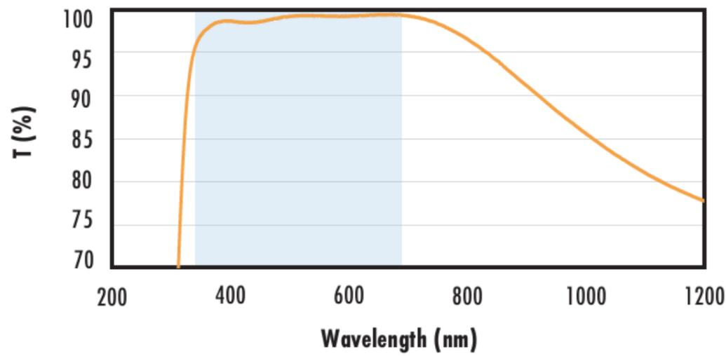
Typical transmission of a fused silica window with VIS-EXT (350-700nm) coating at 0° AOI.
