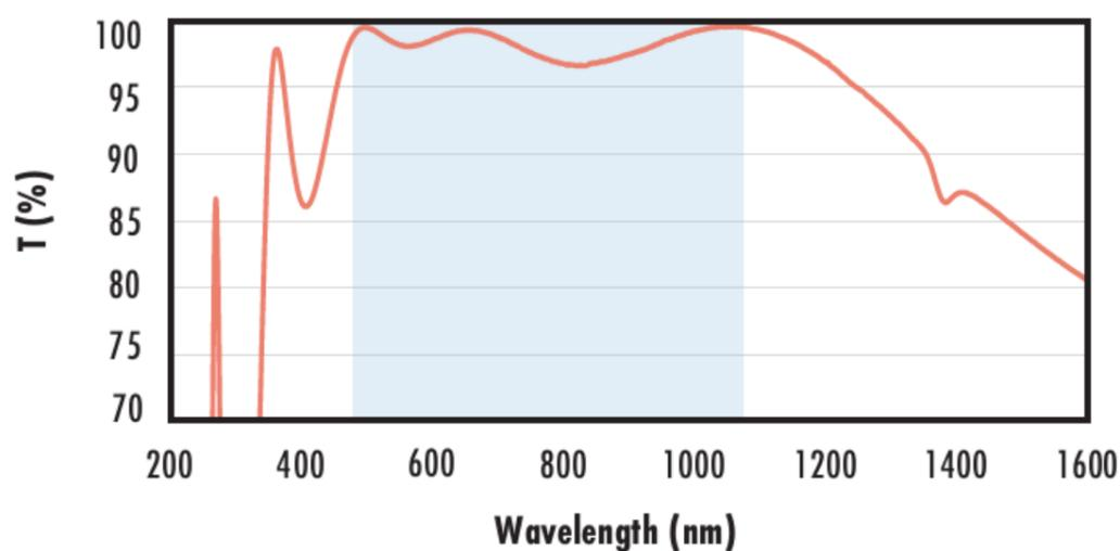
Typical transmission of a fused silica window with YAG-BBAR (500-1100nm) coating at 0° AOI.
