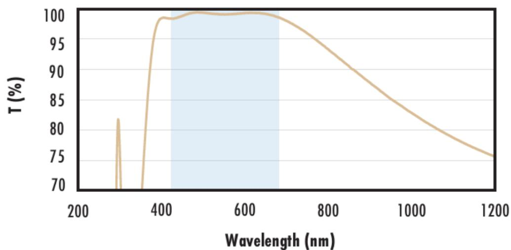
Typical transmission of a fused silica window with VIS 0° (425-675nm) coating at 0° AOI.
