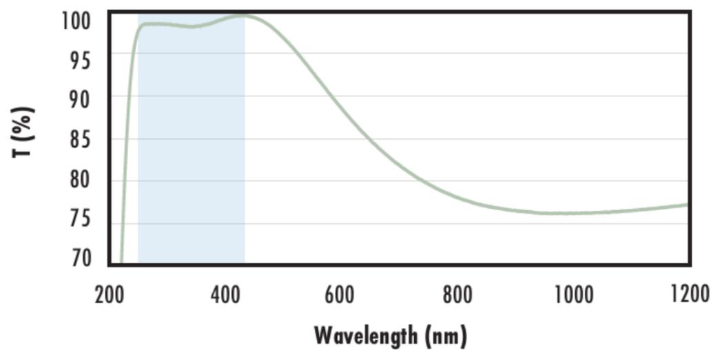
Typical transmission of a fused silica window with UV-AR (250-425nm) coating at 0° AOI.
