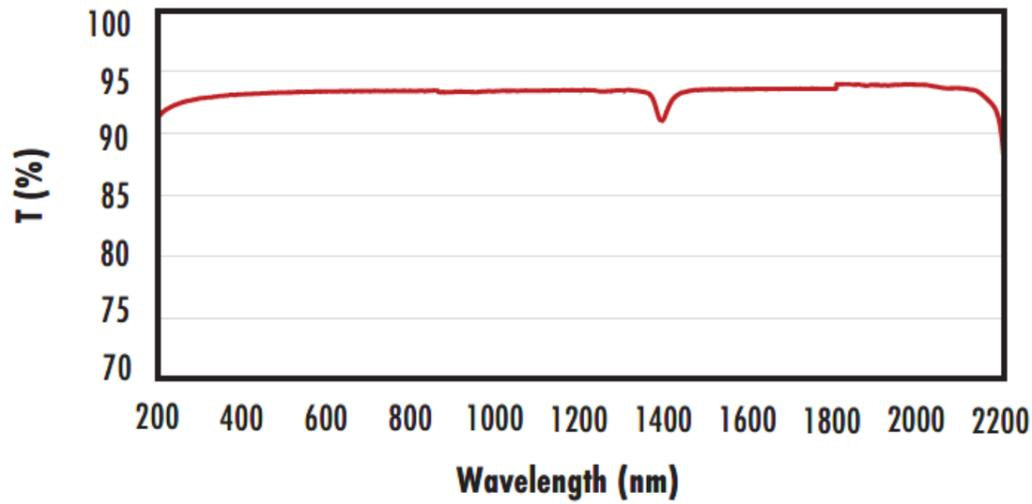
Typical transmission of an uncoated fused silica window across the UV - NIR spectra.
