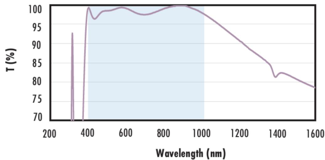
Typical transmission of a fused silica window with VIS-NIR (400-1000nm) coating at 0° AOI.
