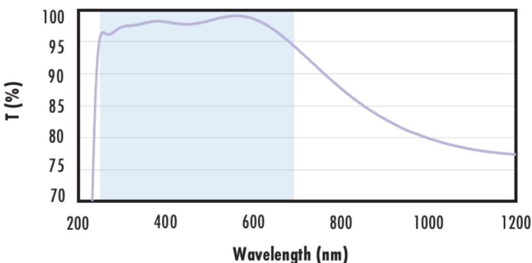
Typical transmission of a fused silica window with UV-VIS (250-700nm) coating at 0° AOI.
