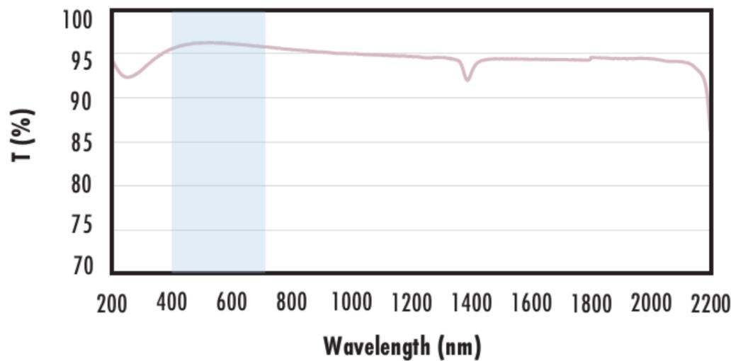
Typical transmission of a fused silica window with MgF<sub>2</sub> (400-700nm) coating at 0° AOI.
