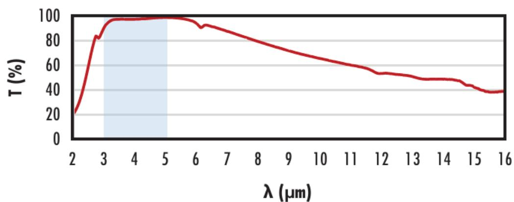
Typical transmission of a 3mm thick Ge window with BBAR (3000-5000nm) coating at 0° AOI.
