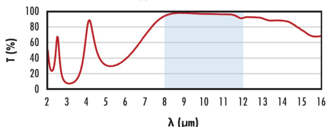
Typical transmission of a 3mm thick Ge window with BBAR (8000-12000nm) coating at 0° AOI.
