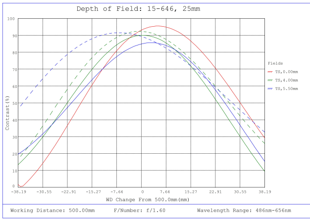
#15-646, 25mm, f/1.6 Cw Series Fixed Focal Length Lens, Depth of Field Plot, 500mm Working Distance, f1.6
