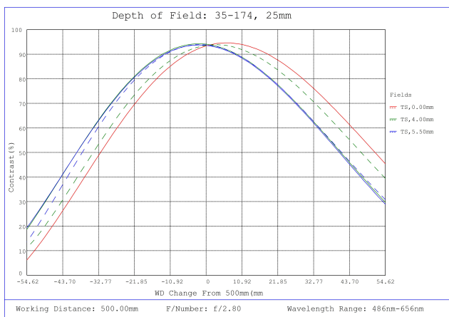
#35-174, 25mm, f/2.8 Cr Series Fixed Focal Length Lens, Depth of Field Plot, 500mm Working Distance, f2.8
