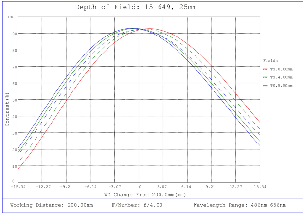
#15-649, 25mm, f/4 Cw Series Fixed Focal Length Lens, Depth of Field Plot, 200mm Working Distance, f4
