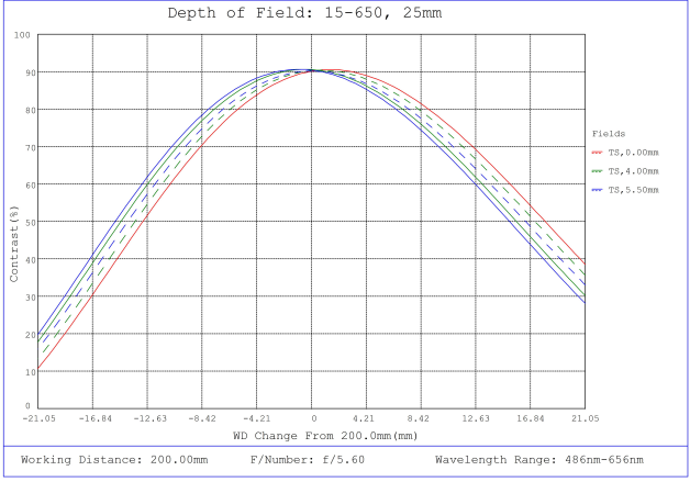
#15-650, 25mm, f/5.6 Cw Series Fixed Focal Length Lens, Depth of Field Plot, 200mm Working Distance, f5.6
