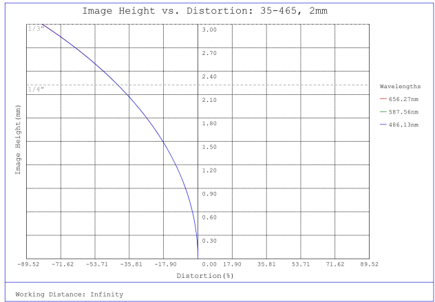
#35-465, 2mm FL f/2.5 IR-Cut, Blue Series M12 Lens, Distortion Plot
