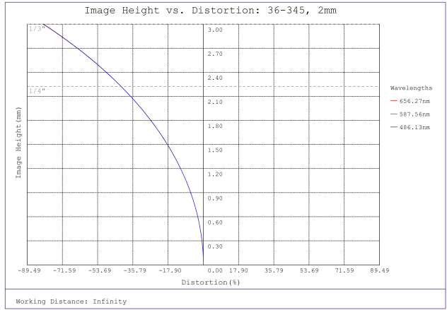
#36-345, 2mm FL f/5.6 Rugged Blue Series M12 Lens, Distortion Plot
