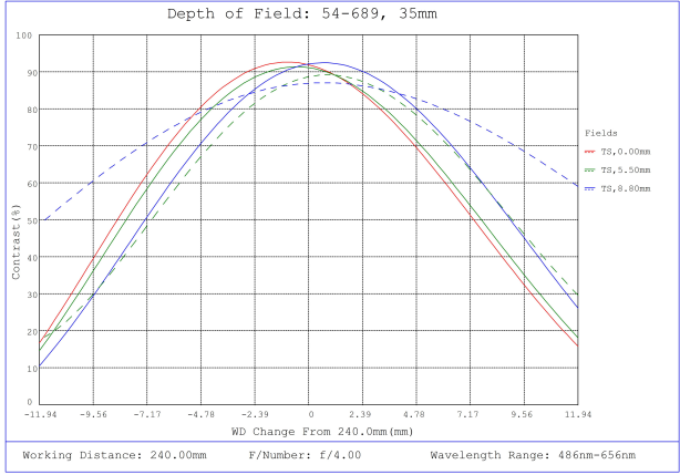
#54-689, 35mm DG Series Fixed Focal Length Lens, Depth of Field Plot, 240mm Working Distance, f4
