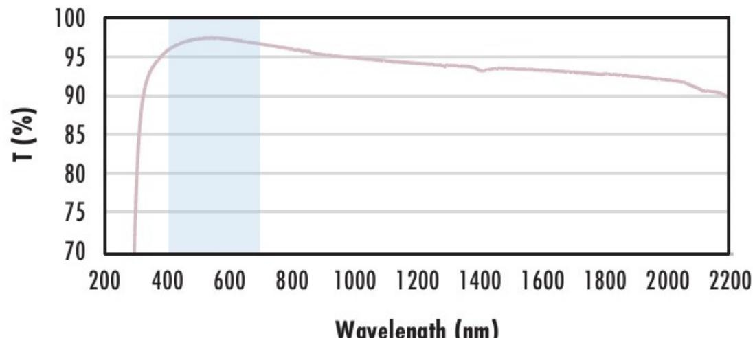
Typical transmission of a 3mm thick N-BK7 window with  $\text{MgF}_2$  (400-700nm) coating at  $0^\circ$  AOI.
