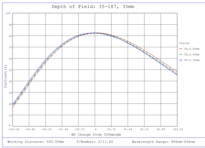
#35-187, 35mm, f/11 Cr Series Fixed Focal Length Lens, Depth of Field Plot, 500mm Working Distance, f11
