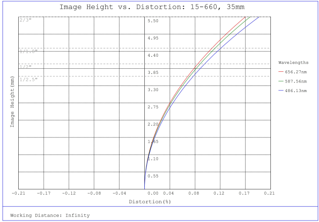
#15-660, 35mm, f/11 Cw Series Fixed Focal Length Lens, Distortion Plot
