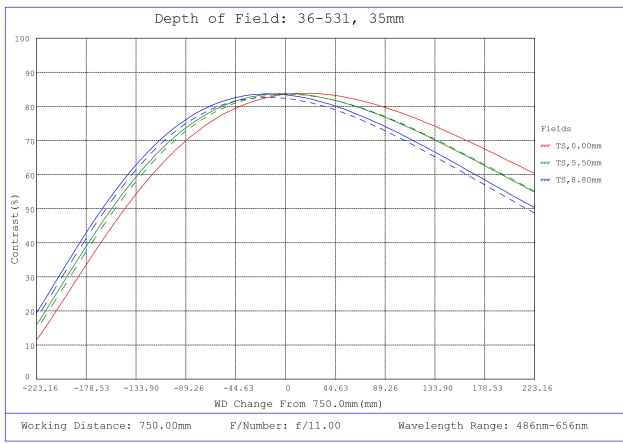
#36-531, 35mm f/11.0, HPr Series Fixed Focal Length Lens, Depth of Field Plot, 750mm Working Distance, f11
