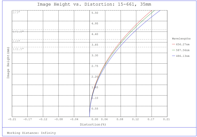
#15-661, 35mm, f/16 Cw Series Fixed Focal Length Lens, Distortion Plot
