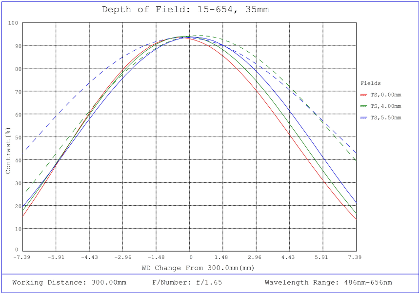
#15-654, 35mm, f/1.65 Cw Series Fixed Focal Length Lens, Depth of Field Plot, 300mm Working Distance, f1.6
