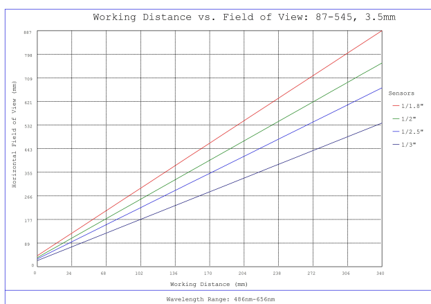
#87-545, 3.5mm, f/2 Ci Series Fixed Focal Length Lens, Working Distance versus Field of View Plot
