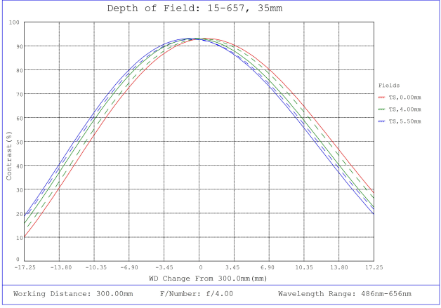
#15-657, 35mm, f/4 Cw Series Fixed Focal Length Lens, Depth of Field Plot, 300mm Working Distance, f4
