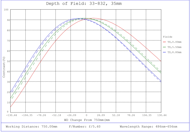
#33-832, 35mm f/5.6, HPi Series Fixed Focal Length Lens, Depth of Field Plot, 750mm Working Distance, f5.6
