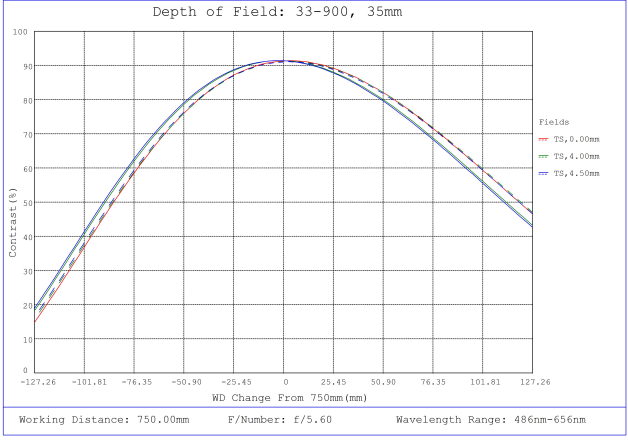
#33-900, 35mm f/5.6, UCI Series Fixed Focal Length Lens, Depth of Field Plot, 750mm Working Distance, f5.6
