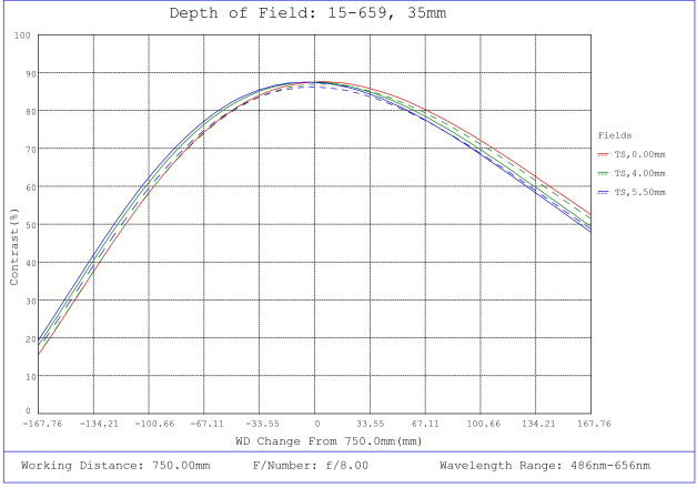
#15-659, 35mm, f/8 Cw Series Fixed Focal Length Lens, Depth of Field Plot, 750mm Working Distance, f8
