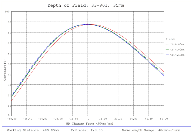
#33-901, 35mm f/8, UCI Series Fixed Focal Length Lens, Depth of Field Plot, 400mm Working Distance, f8
