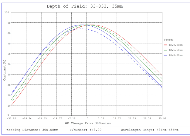
#33-833, 35mm f/8.0, HPI Series Fixed Focal Length Lens, Depth of Field Plot, 300mm Working Distance, f8
