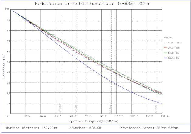
#33-833, 35mm f/8.0, HPi Series Fixed Focal Length Lens, Modulated Transfer Function (MTF) Plot, 750mm Working Distance, f8
