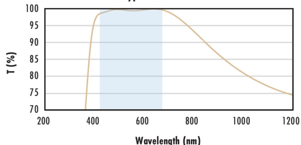
Typical transmission of a 3mm thick N-BK7 window with VIS 0° (425-675nm) coating at 0° AOI.
