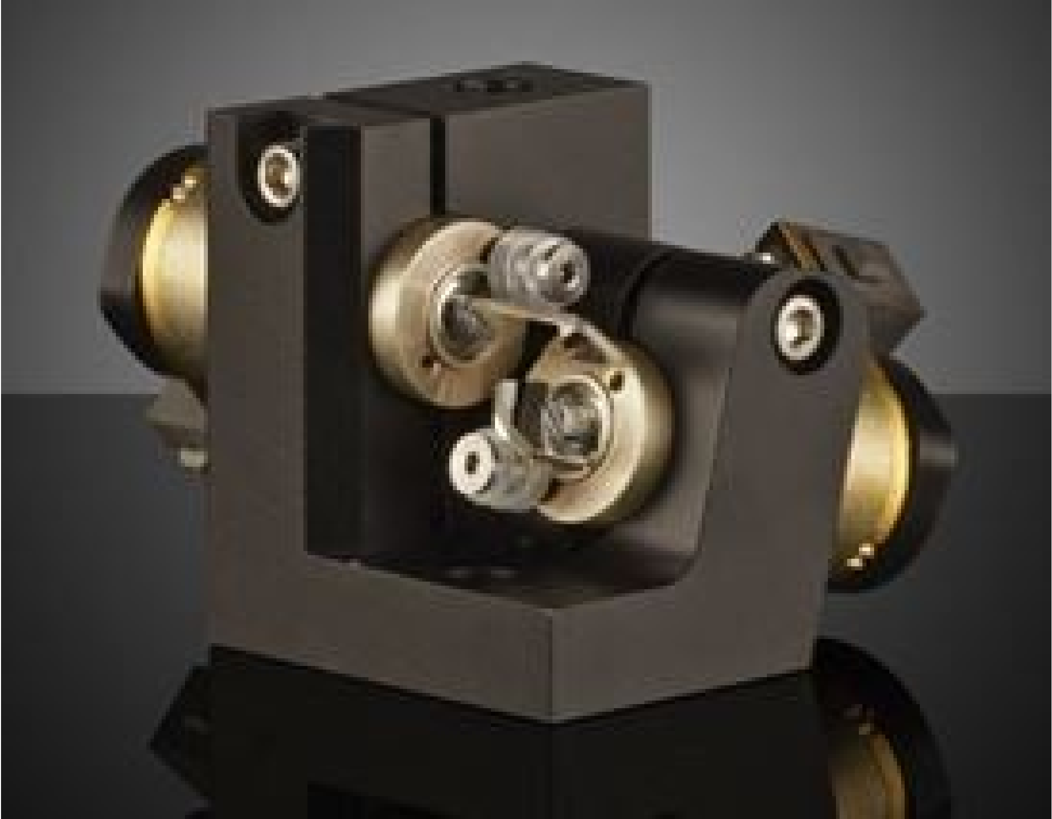
3mm Aperture, Protected Silver, Compact 506 Dual Axis Galvanometer Scanner
