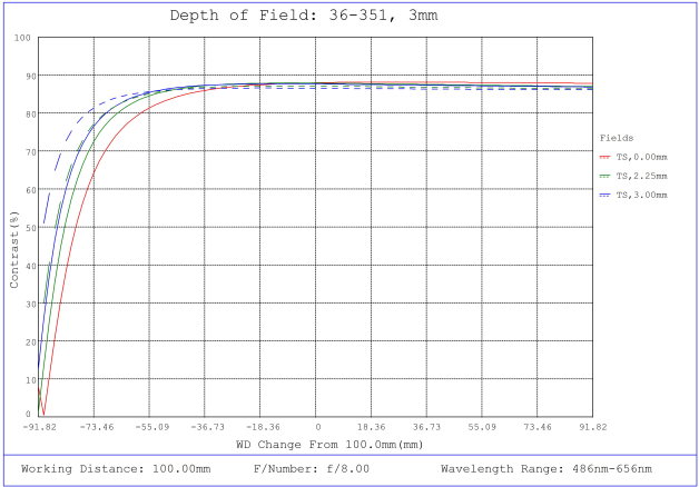
#36-351, 3mm FL f/8, Rugged Blue Series M12 Lens, Depth of Field Plot, 100mm Working Distance, f8
