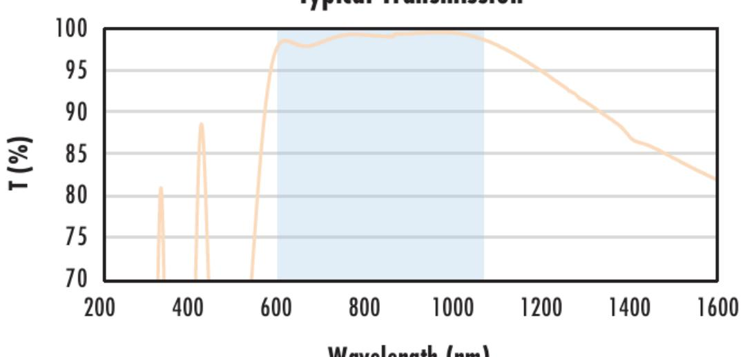
Typical transmission of a 3mm thick N-BK7 window with NIR I (600 - 1050nm) coating at 0° AOI.
