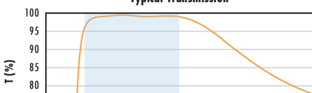
Typical transmission of a 3mm thick N-BK7 window with VIS-EXT (350-700nm) coating at 0° AOI.
