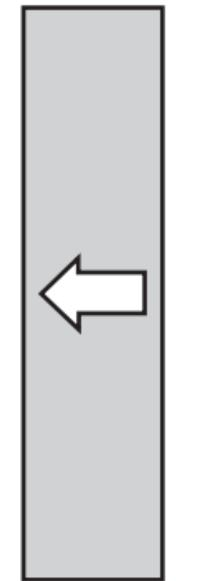
All mounted TECHSPEC® Optical Filters have an arrow on the side of the mount that points to the filter-coated surface for quick reference. Filter oriented such that arrow points to filter coated surface S1.
