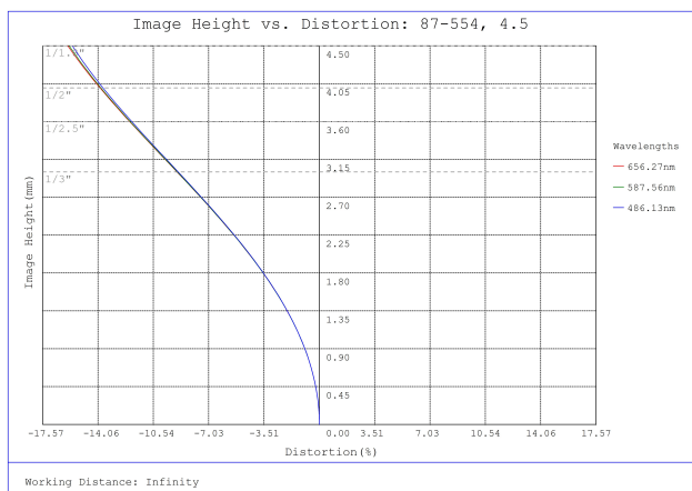
#87-554, 4.5mm, f/5.6 Ci Series Fixed Focal Length Lens, Distortion Plot
