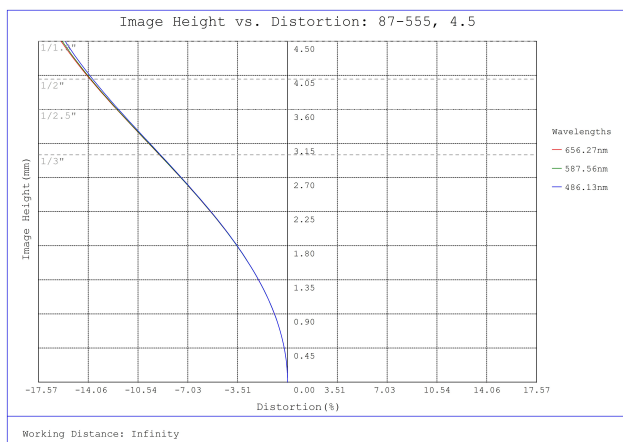
#87-555, 4.5mm, f/8 Ci Series Fixed Focal Length Lens, Distortion Plot
