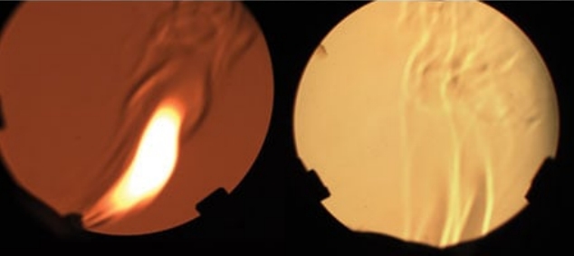
Flame Analysis using 6" Schlieren System
