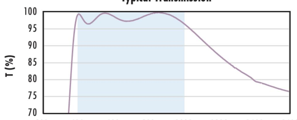
Typical transmission of a 3mm thick N-BK7 window with VIS-NIR (400-1000nm) coating at 0° AOI.
