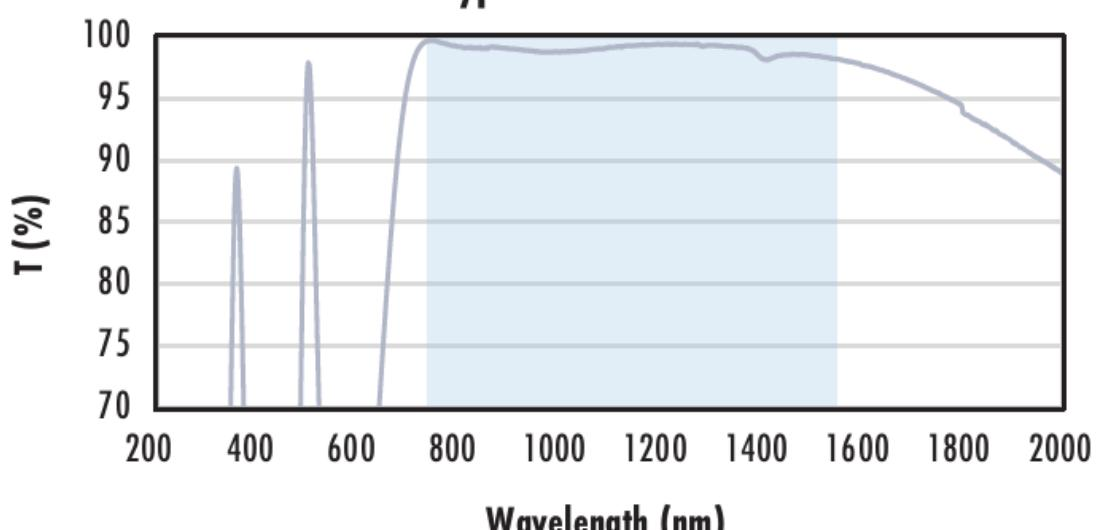
Typical transmission of a 3mm thick N-BK7 window with NIR II (750 - 1550nm) coating at 0° AOI.
